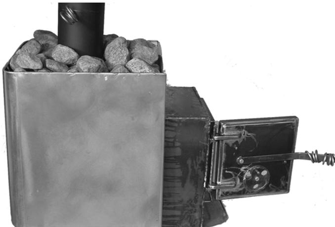
side view with stainless steel heat shield
